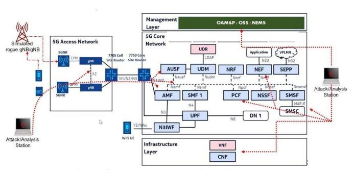
Example attack vectors from RAN access and internal network connectivity
