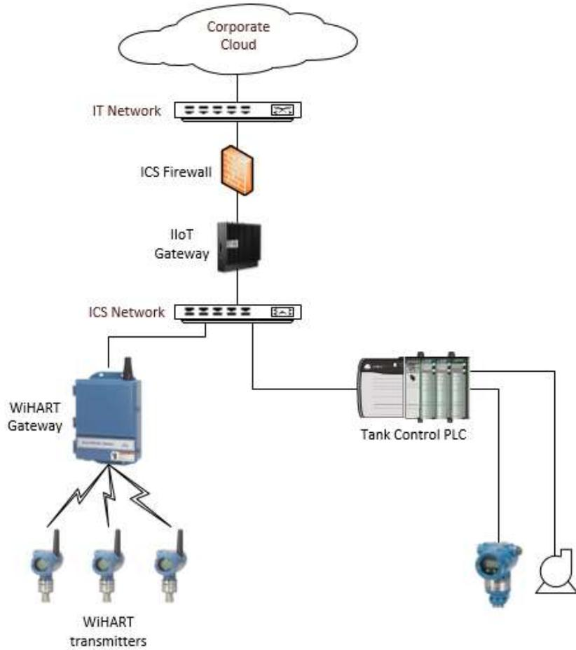
Figure 6: Tank Monitoring Use Case
