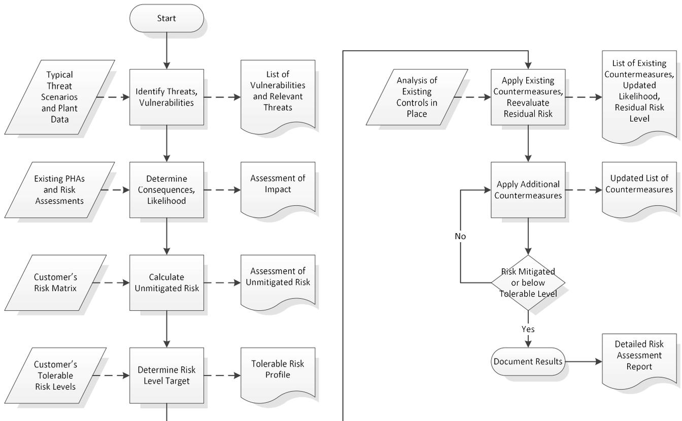
**Figure 9: Cyber PHA Workflow (Adapted from ISA 62443-3-2)**
