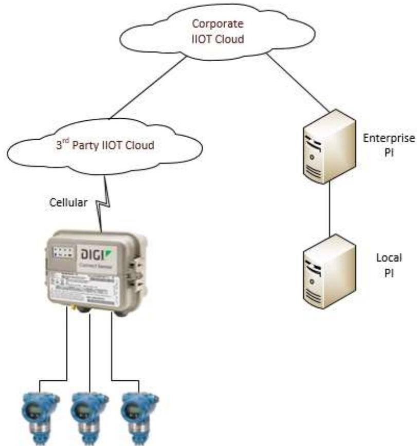
Figure 2: Wellhead Monitoring Use Case
