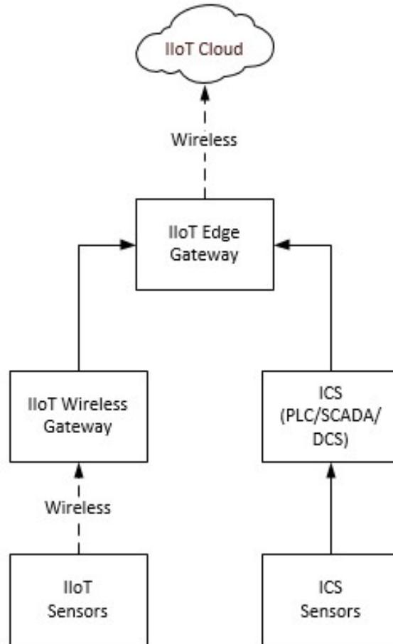
**Figure 3: IIoT Architecture 2**
