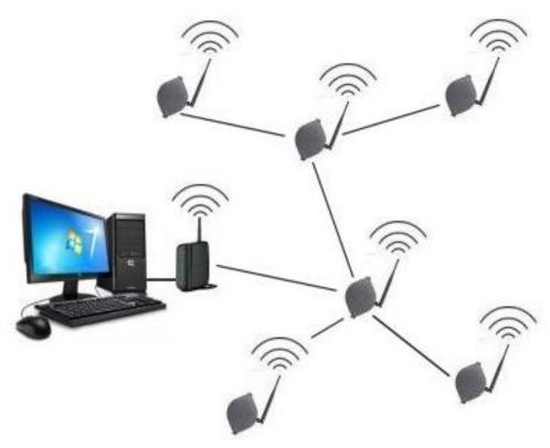
Mesh network transmitter nodes are all able to communicate with each other.
