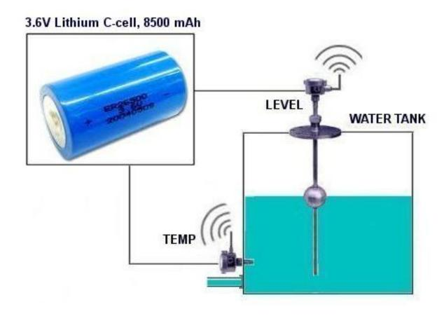
Level and Temperature Transmitter nodes sending data ever 30 seconds (explain cycle-time)
