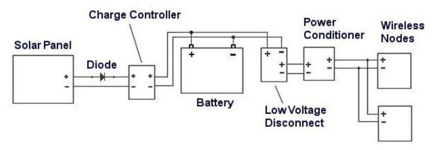
Incorporates a blocking diode you would need to install one.
