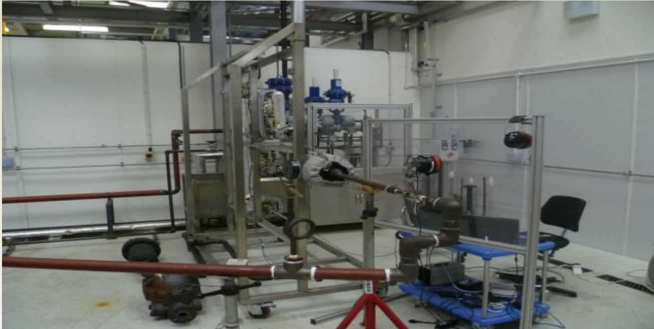
20 - 60 Bar Steam Meter test set up
